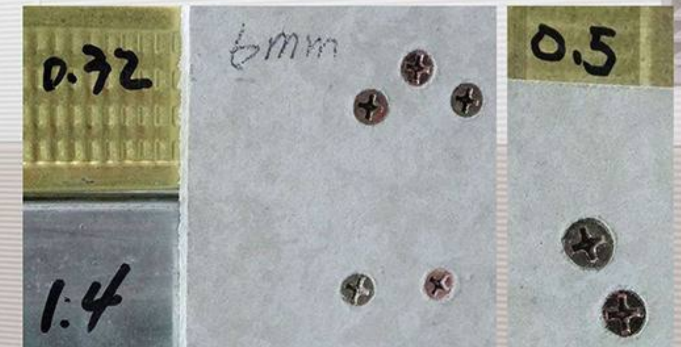
6mm fiber cement board to 0.32, 0.5, 1.4mm steel
